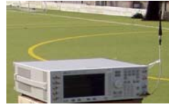
Figure 6 – Signal generator with vertical monopole
