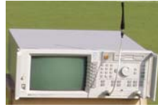
Figure 5 – Network analyzer with vertical monopole
